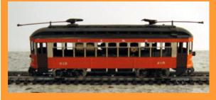
We discovered that we had a second CL&A interurban and decided to convert it into Sand Springs 65. This would require headlights to be installed at both ends and pole towers to be fabricated.
